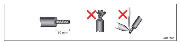
Fig. 3-7: Preparation of the cable
